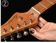
Pull the string through the tuner hole all the way through. At this point, make sure that the ball end of the string reaches the deepest part of the string hole in the tremolo block.
